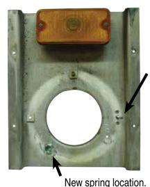
New adjustment screw shown with adjustment plate rivited in new location. MILL SUPPLY, INC. 800-888-5072
