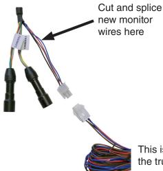
The new monitor comes with a harness that will need 4 wires spliced to your existing system. To make things simpler, you can re-use your existing 4 plug connectors. Just splice your 4 wires into the monitor side, and plug back into the power side of your system. This way you can unplug it at any time.
