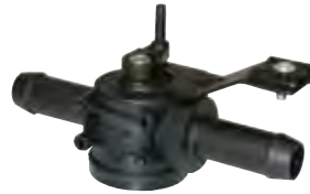
54-591 - Cable operated heater valve. Pull to Close. Remove cable bracket when used with servo actuator. 5/8" outlets. 54-593 - Cable operated heater valve. Pull to Open
