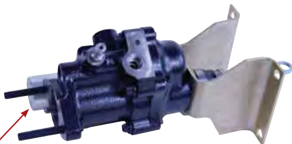
10-901 - Rod extends past the body of unit
