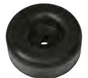
75-250 Engine Cover Rubber Bumper. Recessed for 3/8" bolt. 2-1/2" Dia. x 1"
