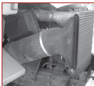
85-387 - Air Filter with Canister, Freightliner MT Models. Uses 85-675 7-3/4" clamp.
