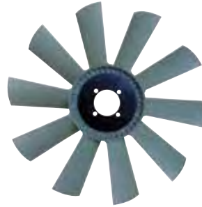
85-173 - 18" Plastic fan that fits original Cummins Clutch. 3-1/4" Center Hole; (4) .335" holes on 3-13/16" centers
