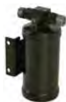
55-140 - Receiver Drier. R-12 or R134A; 2-1/2" Dia x 6-1/4"H. Replaces RV-218370, 47008355
